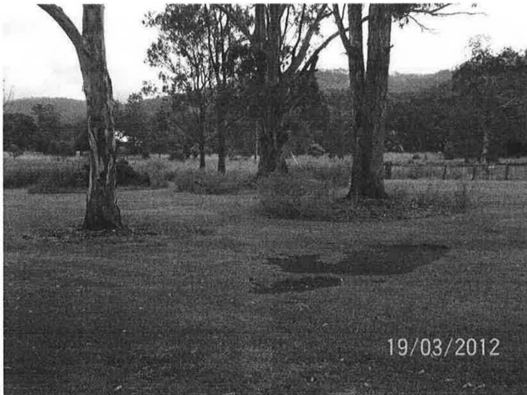
Photo 2 , View of former vehicle parking area and bare patches with surface staining. Soil samples SS05, SS06 and SS07 were collected from the foreground in a transect parallel to the surface staining.
